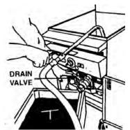
Figure 2.3: Close drain valve
